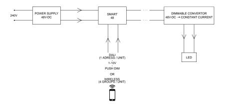
SMART 48: Dimming 48V luminaires or profiles by 2 wires! It collects the power from the 48V power supply and combines it with a DALI, 1-10V or Touch Dim input and sends it to the 48V converter in the luminaire. With the Dimmable Modulator 48V-DC DIM9, dimming can be done by only using 2 wires for both power and dimming.
